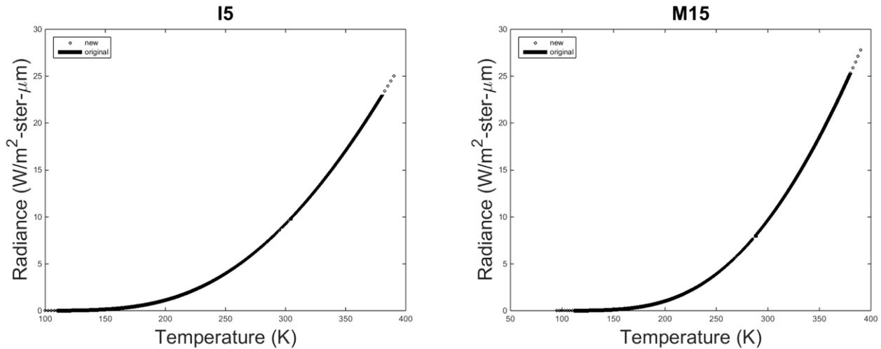
Figure 1. Expanded radiance vs. brightness temperature curves for I5 and M15.
