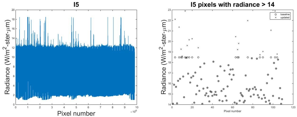
Figure 2. Baseline radiance values for I5 (left). Baseline and updated I5 radiance values pixels with radiance values  $> 14$   $\text{W/m}^2\text{-ster-um}$  (right). The baseline run has radiance values capped at  $18.49 \text{ W/m}^2\text{-ster-um}$  even though the brightness temperature ranges from  $359.0 \text{ K}$  to  $376.2 \text{ K}$ .
